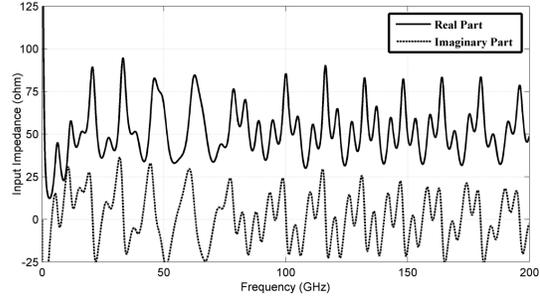
Fig. 6 Input impedance
