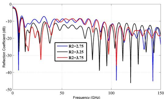
Fig. 3 Reflection coefficients for different values of R2
