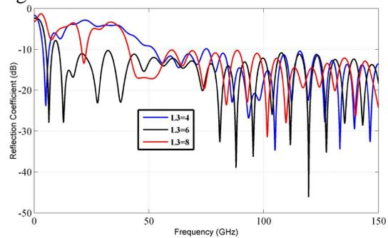
Fig. 4 Reflection coefficients for different values of L3
