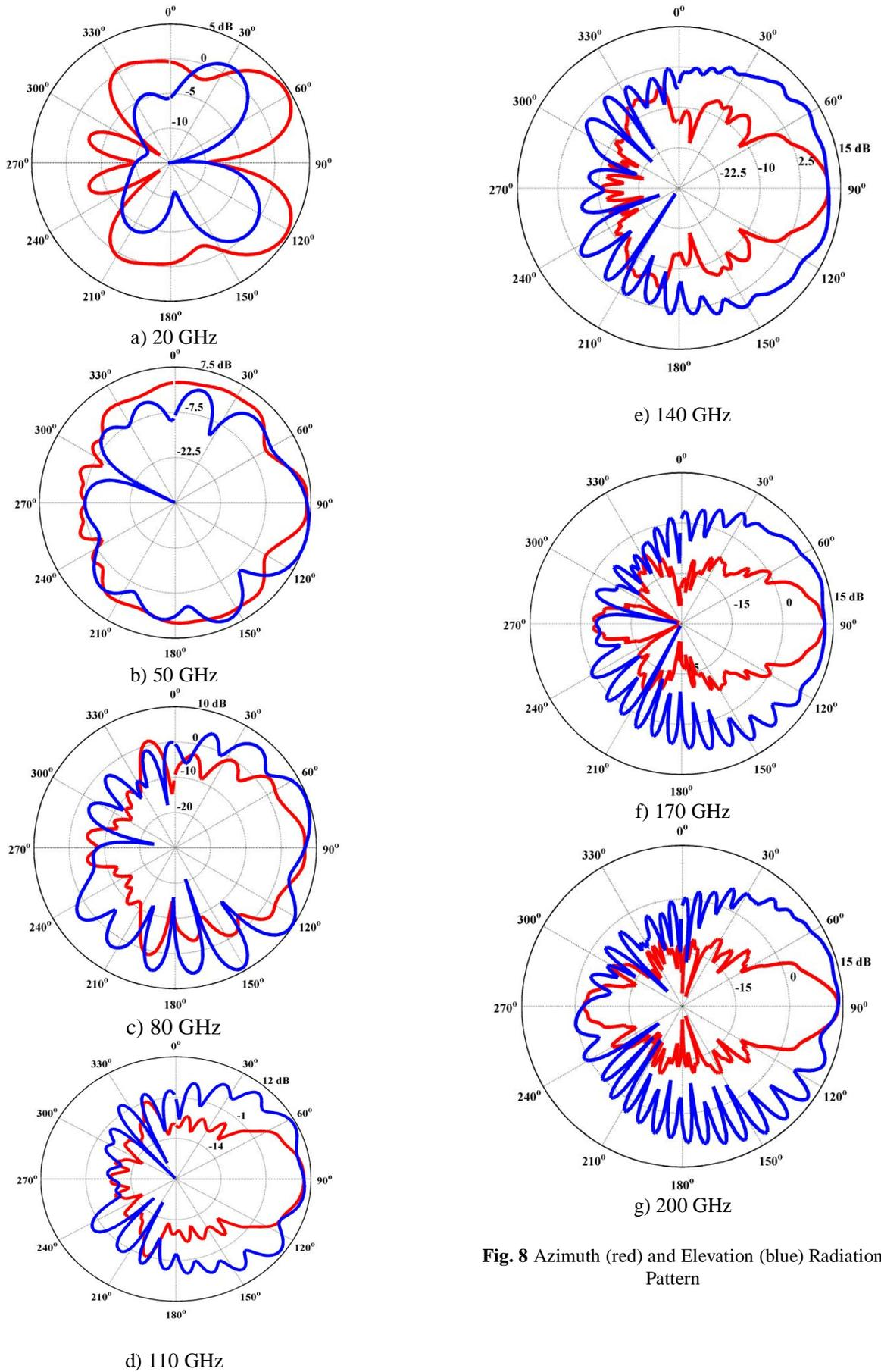
**Fig. 8** Azimuth (red) and Elevation (blue) Radiation Pattern
