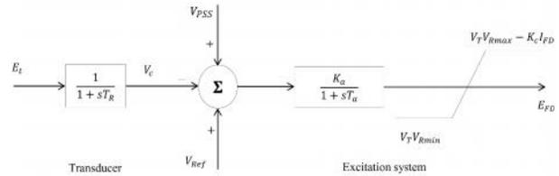
**Fig. 9.** Thyristor excitation system and transducer [2]
