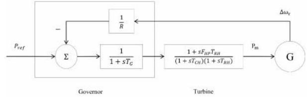
**Fig. 8.** Turbine and speed governor model [1]
