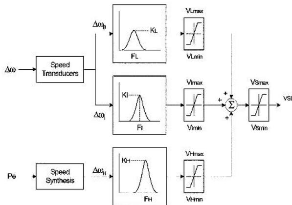
Fig. 10. Conceptual model of multi-band stabilizer (IEEE PSS4B) [2]
