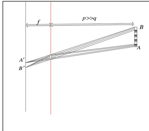
**Figure 1.** image formation for an object in infinite using a lens
