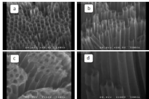
**Fig.2:** SEM images of one dimension TiO<sub>2</sub> nanotubes array with perfect walls (a and b) and three dimension TiO<sub>2</sub> nanotubes array with holes in walls of first nanotubes array (c and d)
