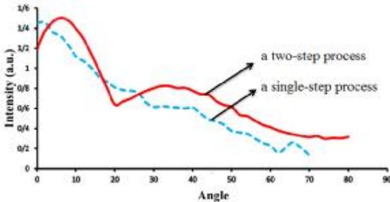
**Fig. 3:** Reflection intensity as a function of angle. Red continuous curve shows reflection spectrum of three dimensional nanotubes array and blue dashed curve shows reflection spectrum of one dimensional nanotubes array. The irradiation wavelength is 330.090 nm
