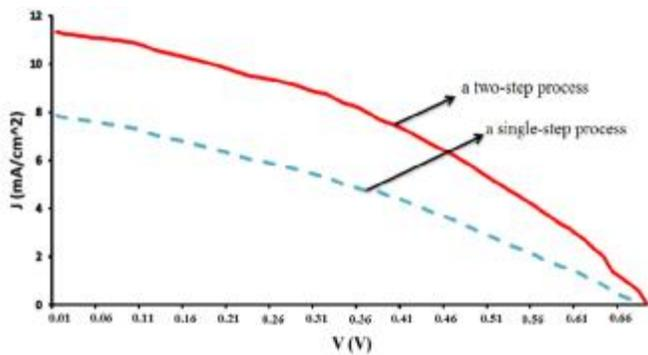
**Fig. 6:** Current density versus voltage of DSSC. Red continuous curve shows behavior of DSSC with a three dimensional TiO<sub>2</sub> nanotubes array as working electrode and blue dashed curve shows same solar cell with a one dimensional nanotubes array as working electrode
