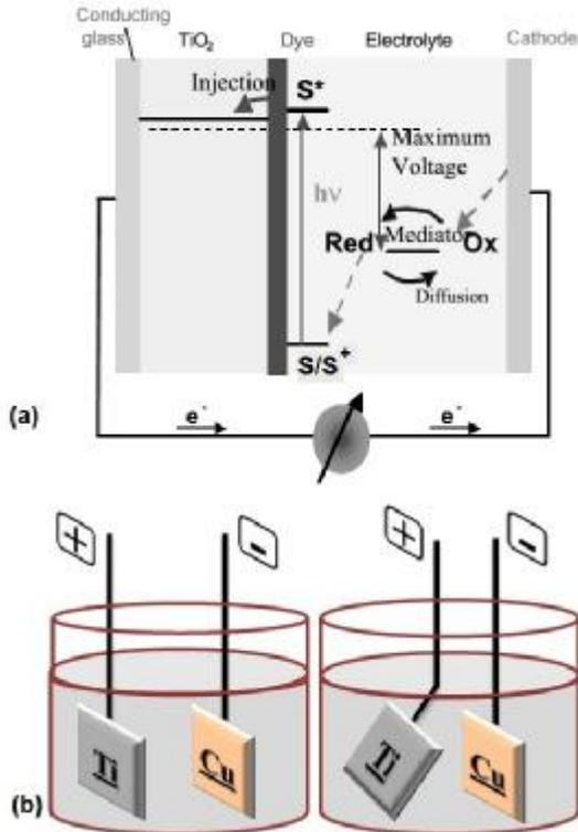
**Fig. 1:** (a) Schematic of a DSSC work condition [7], (b) Two-step anodization process; Anodization by two parallel electrodes as the first step (left) and anodization by electrodes with an angle between them (right).
