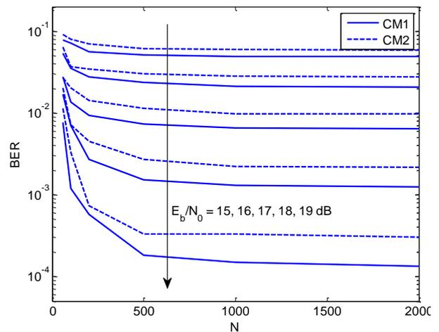
Fig. 2. BER performance at the receiver versus  $N$  with  $2P=20\%$  of  $N$ .
