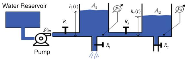
Fig. 1. Two-tank system [6]
