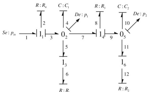
Fig. 2. DHBG model of a two-tank system [6].
