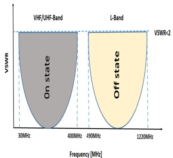
Fig. 1. Frequency operations for the proposed antenna.
