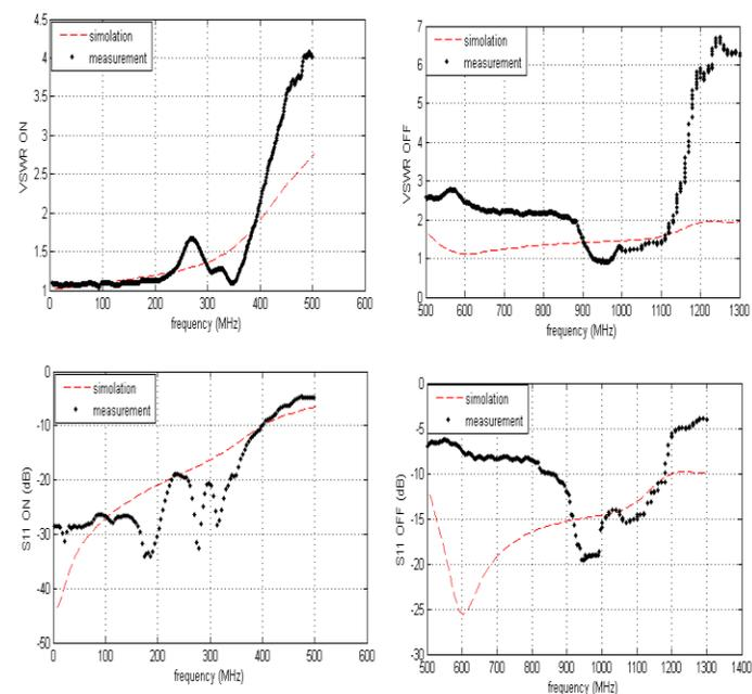
Fig 6. Comparison between simulated and measured reflection coefficient of the presented reconfigurable antenna.
