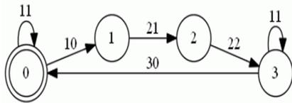
Fig. 19. The feasible supervisor of AGV  $\Sigma_{uo} = \{11\}$ , SUP0
