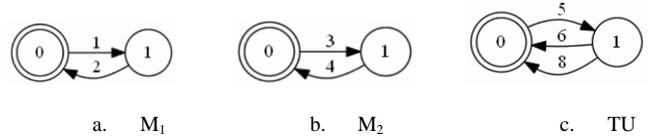
Fig. 6. DES models of M<sub>1</sub>, M<sub>2</sub> and TU
