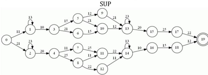
Fig. 13. The feasible supervisor for the guide way  $\Sigma_{uo} = \{13, 23\}$ , SUP<sub>0</sub>
