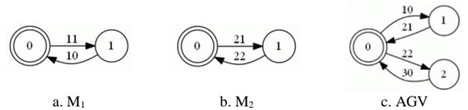
Fig. 15. DES model of each machine and AGV
